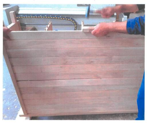
Now put the doors in the two grooves on the front side. First one with handle down, second with handle up.
