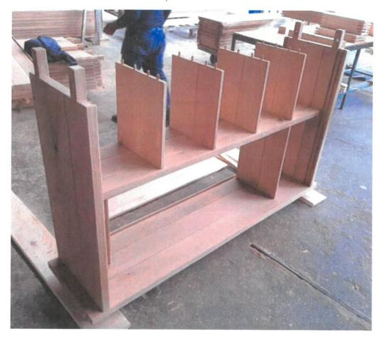
**Step 5.**From behind (where is one groove) put the two back parts. They must be joined with dowels.
