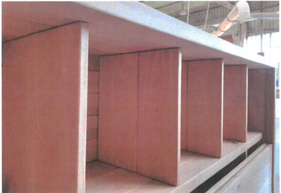
Put the remaining wedges in the holes and be sure that all the angles of the wardrobe are  $90^{\circ}$ .
